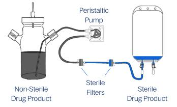
The bulk drug product is typically collected into either a glass mixing vessel or a bioprocess bag. This container will have a sterile connection to attach the drug product to the filling line, and a connection to a sterile filter that allows air to flow out of the bag or vessel as it is filled, without compromising the sterility of the drug product.
