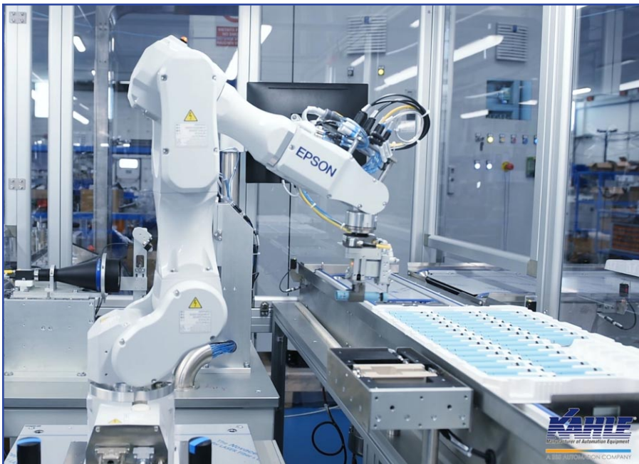
Kahle Automation loading finished pen injectors into trays after assembly.
