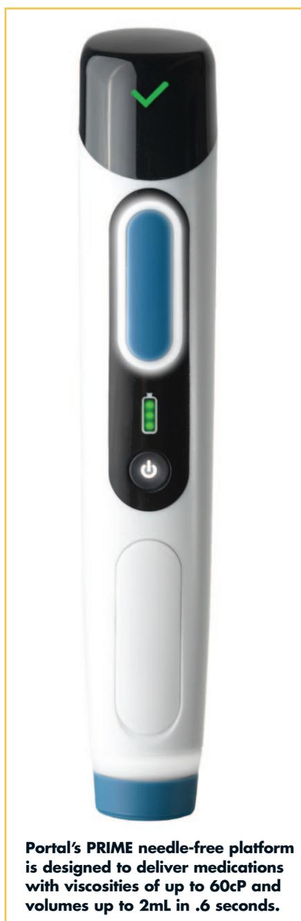
**Portal's PRIME needle-free platform is designed to deliver medications with viscosities of up to 60cP and volumes up to 2mL in .6 seconds.**
