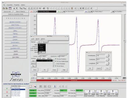
Formation of CM• nitroxide as a function of time in the 2D Field versus Time experiment due to the reaction CMH +  $0_2$ •- -> CM• +  $H_20_2$ . SpinFit and SpinCount modules provide ROS concentration for quantitative EPR analysis at any given time point during the reaction.
