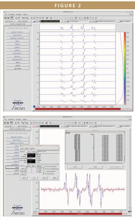
Experimental data (red) and SpinFit simulations (blue) of DMPO radical (superoxide and hydroxyl) adducts in Xanthine/Xanthine oxidase system at a given time in the 2D Field versus Time experiment. Defining the DMPO radical adducts in the SpinFit dialogue by import from library database.
