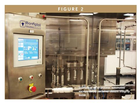
clude vacuum/pressure decay testing, high-voltage leak detection, and methods that utilize a laser to analyze the head space of a filled unit. There is also an instrument by Heuft<sup>™</sup> called the Syringer<sup>®</sup> that uses x-ray pulses to identify syringes with bent needles and needles that puncture the caps. Vacuum/pressure decay, headspace analysis, and high-voltage leak detection methods are more common and are easily attached to a production line for 100% inspection (Figure 2).
