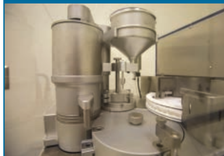
Xcelience's liquid-fill services use Capsugel's CFS 1200™ system for filling and sealing.
