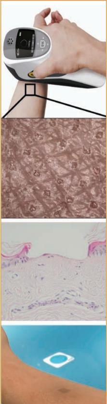
Pantec's P.L.E.A.S.E. hand-held laser device creates aqueous micropores in the epidermis to deliver drugs painlessly.
