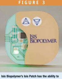
Isis Biopolymer's Isis Patch has the ability to transport up to three drugs per patch and is fully programmable for customized delivery.
