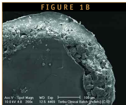
SEM of pellets (A) surface morphology (B) cross-section of the pellet showing salt core, modulating layer (EUDRAGIT® NE), terbutaline sulphate layer and controlled-release layer (EUDRAGIT® RS)
